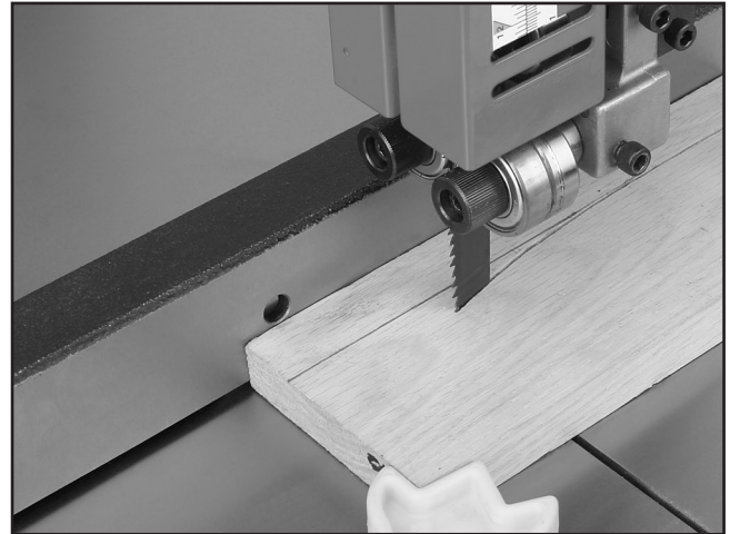
Figure 67. Blade leading away from line of cut.
